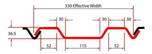
The overlapping trench sheeting profile is produced in S275JR steel with a thickness of 3.4mm. These are designed primarily for construction work and temporary groundworks.
